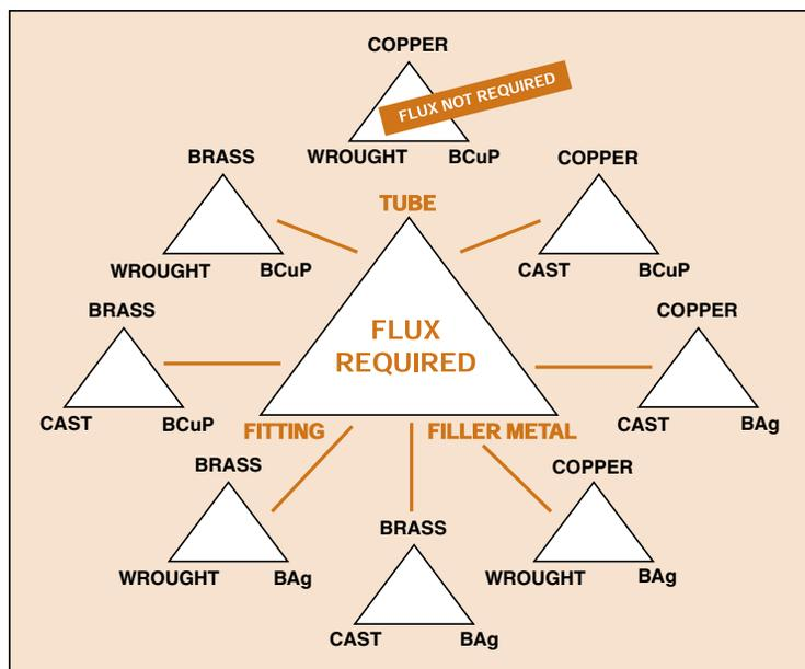
Triangles, denoting when to use flux, are surrounded by tube type, fitting type and brazing filler type.
