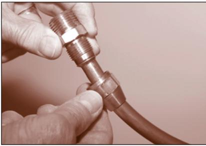
**FIGURE 28: Flare Fitting/Flared Joint During Assembly**
