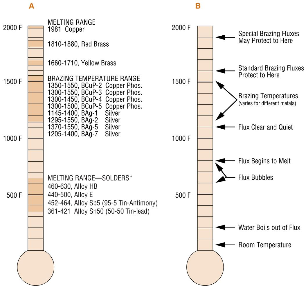
**NOTE:** \* Melting ranges of solder alloys are in accordance with the alloy manufacturers' product information and may not match the melting ranges shown in ASTM B32.
