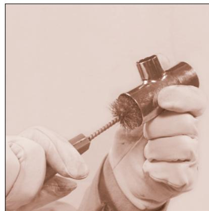
FIGURE 17: Cleaning: Fitting Brush
