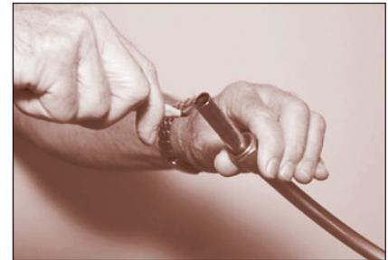
**FIGURE 30: Reaming Prior to Flaring the Tube End**
