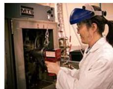
From the McGill website (2006): Hee Eon Park, first-year postdoc in Chemical Engineering, works on a high-pressure sliding plate rheometer, the only instrument of its kind in the world.
