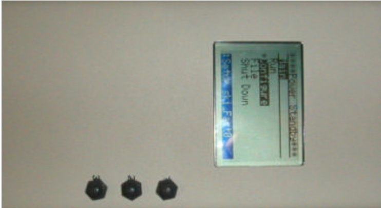
Figure 2. The GEM-2 console showing the push buttons and command menu.
