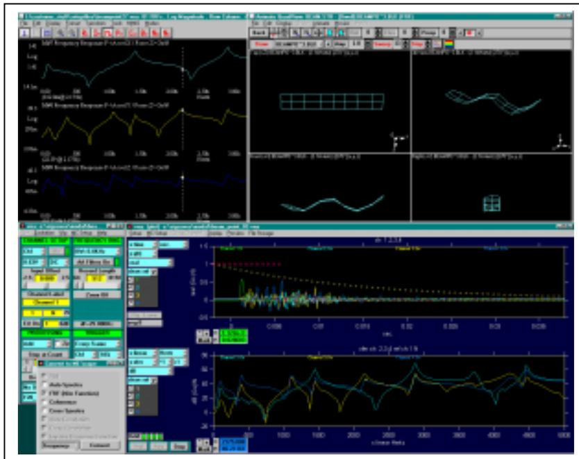
*Figure 7-1 An example of a SigLab modal test. The structure used was a free-free aluminum beam approximately 7” in length, 1.5” wide and 1/8” thick. A triaxial accelerometer was mounted at 1 end. Using VNA, with a modal impact hammer to excite the beam, 3 FRF measurements were made at each of 27 points on the beam. These were then imported into ME’scope and used to animate a wireframe model of the beam.*
