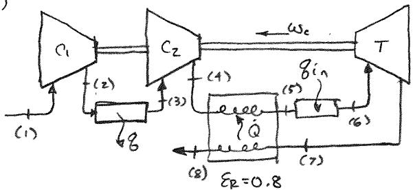
$$\dot{W}_{\text{net}} \quad r_p = 4.5 \quad \eta_t = \eta_c = 0.80 \quad \epsilon_R = 0.80$$
