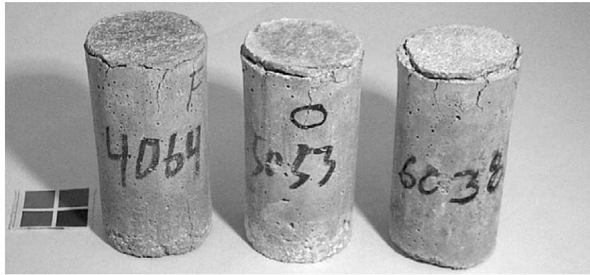
Fig. 1. From left to right: 0.40, 0.50, and 0.60 w/c mortar cylinders after 84 days in cold \text{MgCl}_2 brine. Cylinder dimensions are 50 mm in diameter and 100 mm in height.
