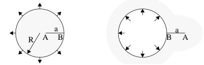
**Numerical Model**: The circular boundary was represented by indirect BEM with force singularity. The crack was modelled by displacement discontinuity. The crack was modelled by 33 linear lagrange elements and the circular boundary by 33 linear lagrange element. Discontinuity in density function at point B was permitted.
