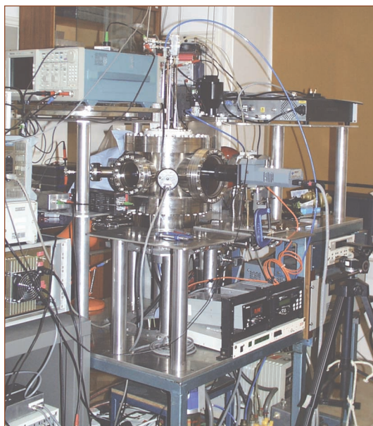
Figure 7. DARBS application. The system interacts with plasma deposition equipment through sensors and actuators. (Photo by Lars Nolle.)
