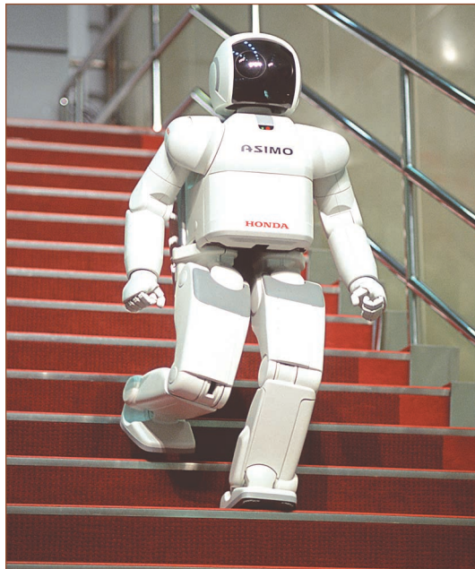
Figure 2. Honda's Asimo robot descending a flight of stairs. Asimo has 16 flexible joints with a four-processor computer to control its balance and movement, but its intelligence is limited. (Source: Honda. Used with permission.)
