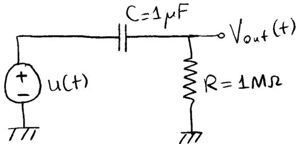
Where  $u(t)$  is a step function,  $R = 1 \text{ M}\Omega$ ,  $C = 1 \mu\text{F}$  (fixed during the test)
