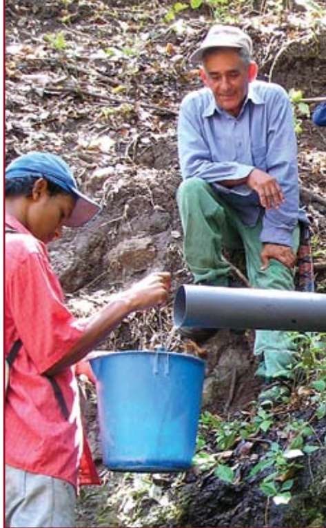
At left, technicians and local residents of a small watershed take a streamflow measurement during the height of the dry season. At right, ENACAL engineers and technicians perform a pumping test in one of the wells used in Peace Corps Master's International student Essa Gross's study.
