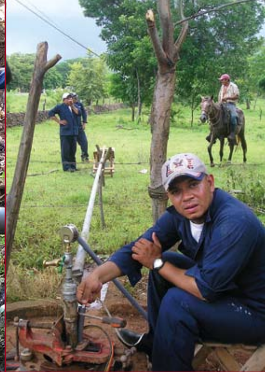
At left, technicians and local residents of a small watershed take a streamflow measurement during the height of the dry season. At right, ENACAL engineers and technicians perform a pumping test in one of the wells used in Peace Corps Master's International student Essa Gross's study.
