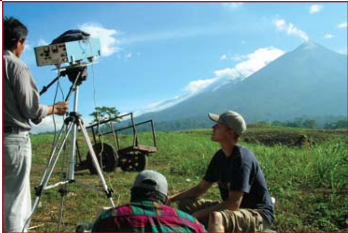
Below: Guatemalan scientists (INSIVUMEH) and Peace Corps Master's International John Lyons conducting gas emission measurements at Fuego volcano as part of routine volcanic activity monitoring.
