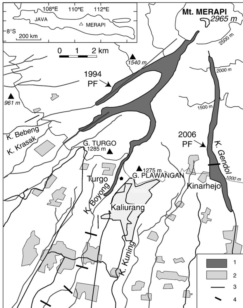
Fig. 6. Studied area on the southern flank of Merapi volcano. 1: block-and-ash flow deposits; 2: village; 3: road; 4: retention dam.
