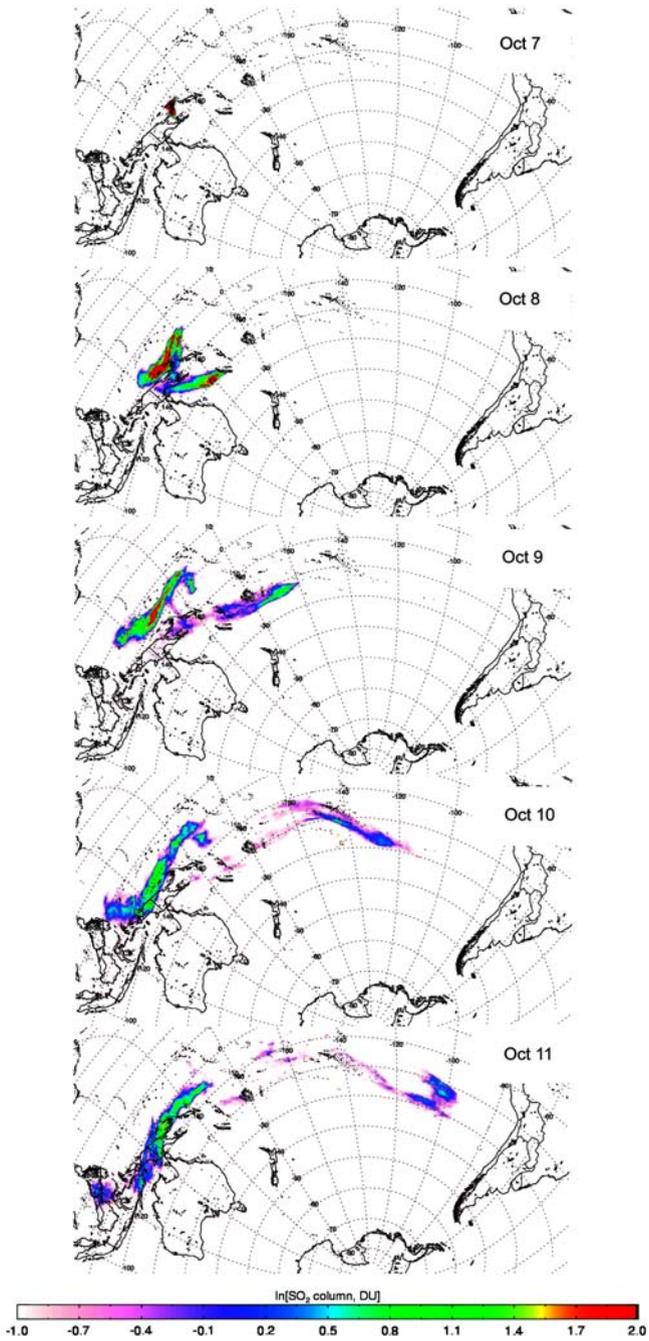
**Fig. 4** Sequence of OMI SO<sub>2</sub> retrievals for the first 5 days of atmospheric residence of the Rabaul volcanic cloud in October 2006 (Oct 7–11). SO<sub>2</sub> VCDs are shown using a log scale
