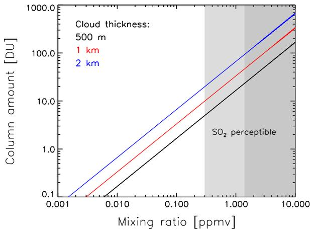
**Fig. 6** Estimated SO<sub>2</sub> mixing ratios corresponding to measured VCDs in a volcanic cloud of variable thickness at 10 km altitude. SO<sub>2</sub> is usually perceptible by humans above ~0.3–1.4 ppm (IVHHN 2007)
