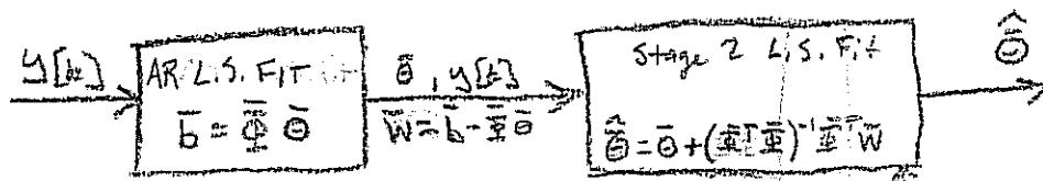
Effectively an ARX fit with error from stage 1 functioning as an input.
