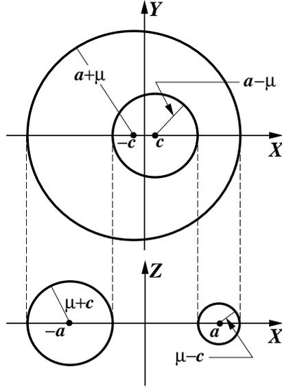
Fig. 2. Longitudinal and latitudinal principal circles of a Dupin cyclide
