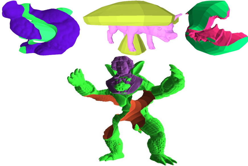
Fig. 5. Some shapes produced by Alg. 2. From left to right: \text{Bunny} \cap \text{Knot} , \text{Pig} \cup \text{Mushroom} , \text{Beethoven} \cap \text{Goblet} , (\text{Armadillo} \cup \text{Beethoven}) \cap \text{Knot}
