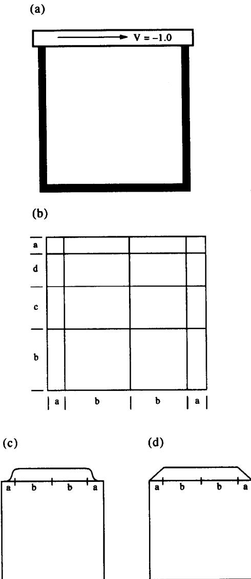
Fig. 14. Lid driven cavity: (a) schematic; (b) 16 element graded mesh; (c) cubic boundary conditions at the top corners; (d) linear boundary conditions at the top corners.
