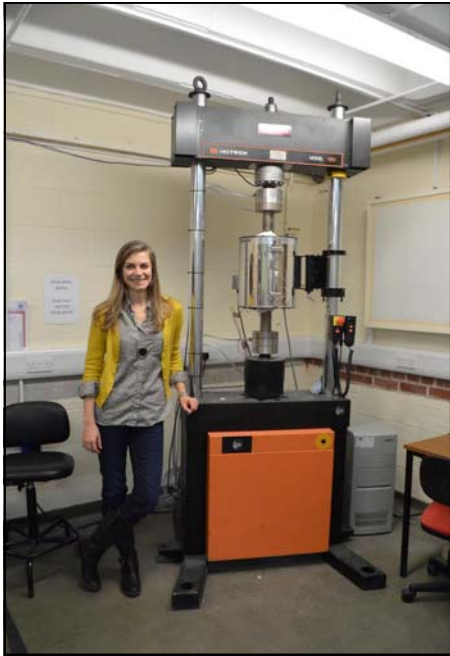
Above. Lauren using a high temperature, high pressure uniaxial press to test volcanic rock at the University of Liverpool, UK.
