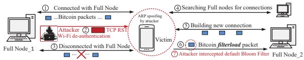
Figure 2: The initiation of the retransmission of filterload messages via TCP reset and Wi-Fi de-authentication attacks.
